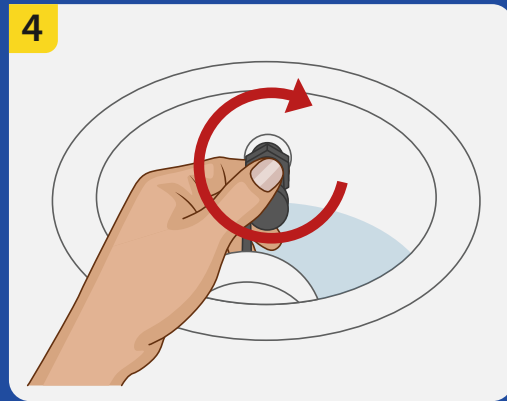
Install float valve, hand tighten so not over tighten.
